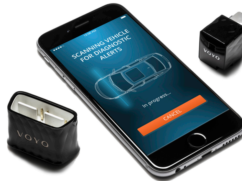
■ Cloud connectivity and data sharing promise consumers an entirely new range of convenience, safety, productivity and infotainment options. Voyomotive is helping to break this ground with Voyo, an advanced telematics system that connects a vehicle’s OBD-II port to the cloud, allowing vehicle owners to monitor and control an array of vehicle functions from virtually anywhere via their mobile devices.
