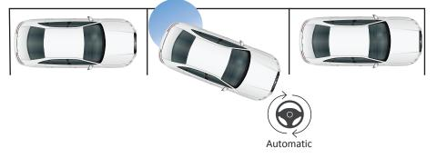
■ Automated PAS exhibits a higher degree of vehicle integration than passive systems, helping to steer a car into parking spaces. Autonomous valet takes things even further, essentially autopiloting the vehicle. Expensive and complex, such systems will almost certainly remain in OEM hands for the foreseeable future.
