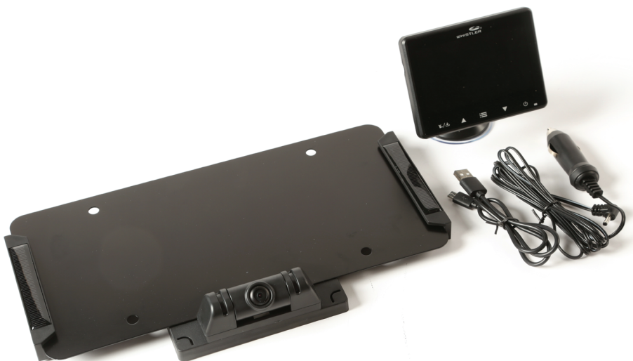
■ Whistler's WBU-900 Wireless Digital Backup Camera offers consumers a novel alternative to costly installation. Like other backup cameras, it attaches to the rear license plate, but it transmits images wirelessly, recharging itself with built-in solar panels.
